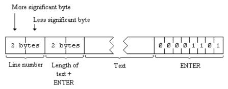
Note that, in contrast with all other cases of two byte numbers in the Z80, the line number here is stored with its more significant byte first: that is to say, in the order that you write them down in.
