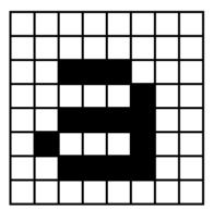
The character position also has associated with it two colours: the ink, or foreground colour, which is the colour for the black dots in our square, and the paper, or background colour, which is used for the white dots. To start off with, every position has black ink and white paper so writing appears as black on white.
